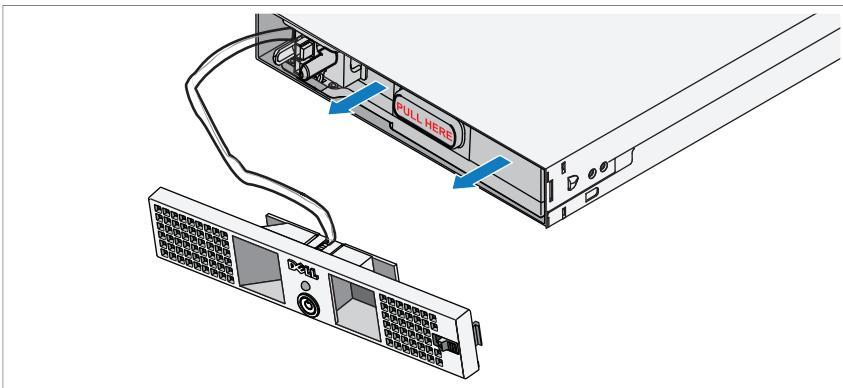
Pull the battery out of the power module.
