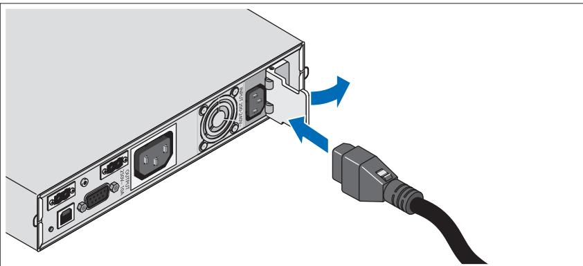
Open the spring-loaded interlock cover for the input connector and connect the power cable to the BPS.
