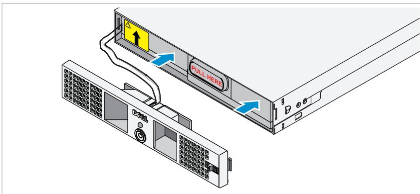
Align the battery with the power module and reinsert the battery. Ensure that the battery is fully seated in the power module. If the battery is not fully inserted into the power module, the battery front cover will not close properly.
